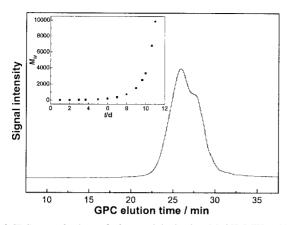
Fig. 2 GPC trace of polymer 3 after precipitation into MeOH (MW = 9900; PDI = 1.9). The inset shows polymer growth as a function of time for a polymerisation run at  $60\,^{\circ}$ C.
