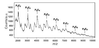
**Fig. 1** MALDI-TOF mass spectrum of the polymerisation mixture showing the incorporation of the porphyrin (P) and epoxide (E) monomers. The peaks at lower (higher) mass of each major peak correspond to the loss (addition) of one epoxide unit.
